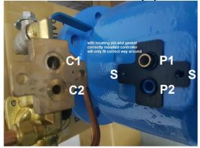
Place the Pipework Assembly onto the gasket by Hand, making sure P1 insert fits into C1, and P2 into C2. It should only fit one way around.
